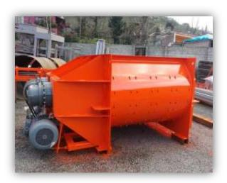
THE MIXER IS PROVIDING HOMOGENEOUS MIXING OF AGGREGATE. MOTOR POWER IS 2  $\times$  45 kw. HANDLE SYSTEM IS AS REPLACEABLE DESIGNED. BY THE PALLETS HANDLE - BY BASE WEAR PLATES AND BY ABRASION SHEET METAL HARDOX / ST 52 - A1 QUALITY MATERIAL IS USED.
