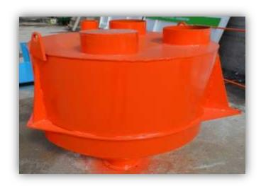
THIS DEVICE IS PROVIDING THE WEIGHING AND SENDING MATERIALS SUCH AS CEMENT – COLOR PIGMENT AND ADDITIVES TO THE MIXER. THE WEIGHING IS PROVIDED WITH 3 PIECES OF 1.000 Kg. LOADCELL. WAM BRAND ACTUATOR WITH VALVE AND MICRO SWITCH IS USED. **WATER**; WILL BE ADDED TO THE MORTAR VIA WEIGHING HOPPER OR DIGITAL WATER METER. THE CAPACITY OF ADDITIVE WEIGHING HOPPER IS 100kg. COLOR PIGMENT WEIGHING HOPPER IS 150kg.
