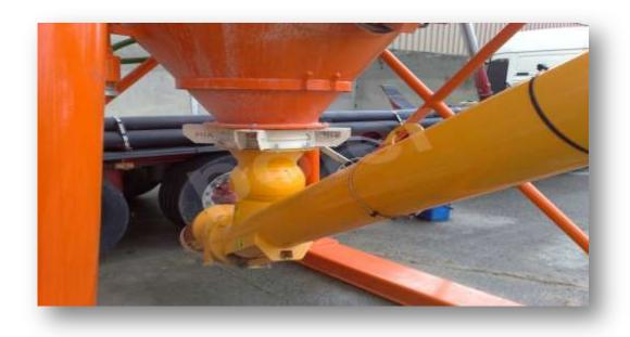
TAKES THE NEEDED CEMENT FOR MORTAR FROM THE SILO TO FEED THE WEIGHING CONVEYOR. WAM BRAND. 8'(\$\psi^2\$19 mm) MOTOR POWER IS 9,2 Kw. SILO CONNECTION POINT IS MOVABLE.
