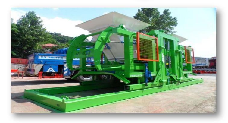
MORTAR UNIT BASE PLATES: HARDOX 450
