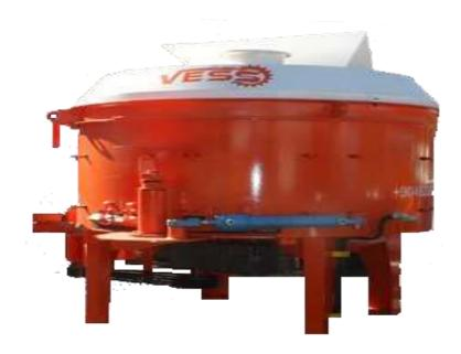
THE MIXER IS PROVIDING HOMOGENEOUS MIXING OF AGGREGATE. MOTOR POWER IS 22 kw. SLEEVE SYSTEM IS AS REPLACEABLE DESIGNED. BY THE PALLETS HANDLE - BY BASE WEAR PLATES AND BY ABRASION SHEET METAL HARDOX / ST 52 - A1 QUALITY MATERIAL IS USED.
