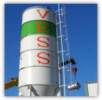
CEMENT STORAGE EQUIPMENT. BESIDES ARE WALKING STAIRS FOR EMERGENCIES. THE CAPACITY IS 200 TON AND REPLACEABLE CARTRIDGE FILTER IS PROVIDED. THERE IS ALSO 2 PIECES LEVEL MEASURING CENSOR PROVIDED AND SAFETY VALVE TO PREVENT OVERFILLING. TO DISCHARGE THE SILO INTO THE CEMENT FEEDING SCREW THERE IS A WAM BRAND VALVE. MANUFACTURED AS STEEL CONSTRUCTION USING 5/6 mm SHEET METAL.
