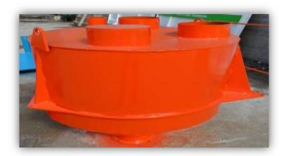
THIS DEVICE IS PROVIDING THE WEIGHING AND SENDING MATERIALS SUCH AS CEMENT – COLOR PIGMENT AND ADDITIVES TO THE MIXER. THE WEIGHING IS PROVIDED WITH 3 PIECES OF 2000 Kg. LOADCELL. WAM BRAND ACTUATOR WITH VALVE AND MICRO SWITCH IS USED. **WATER**; WILL BE ADDED TO THE MORTAR VIA WEIGHING HOPPER OR DIGITAL WATER METER. THE CAPACITY OF ADDITIVE WEIGHING HOPPER IS 400kg. COLOR PIGMENT WEIGHING HOPPER IS 300kg.
