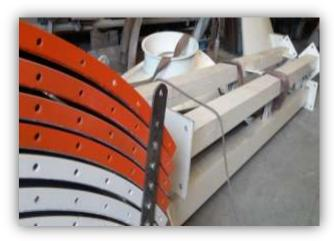
FOR EASY SHIPMENT; OPTIONALLY THE SILO CAN BE MANUFACTURED AS DEMOUNTED (BOLTED)
