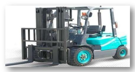
IS USED FOR THE TRANSPORTATION OF THE STACKED PALLETS TO THE DRYING ROOM AND TRANSFERS THE PALLETS TO THE REAR EMPTY PALLET UNLOADER ROBOT, COMING FROM THE DRYING ROOM.TRANSFERS ALSO THE PRODUCTS READY FOR SHIPMENT TO THE STOCKING AREA WHICH ARE ALREADY PACKED DIESEL – ISUZU MOTOR 3 TON CARRYING CAPACITY AND h; 4.20 MT LIFTING CAPABILITY.
